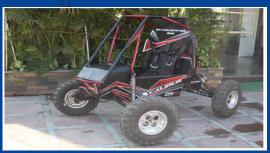
Team Aryans of Govt. College of Engineering Aurangabad has a good legacy in making ATV's. Vehicle includes different systems as rollcage, suspension, steering, transmission, drivetrain, brakes, data acquisition, etc. Static structural analysis and topology optimization of components is performed on different
